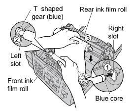
Turn the "T" shaped gear (blue) in the direction of the arrow.
